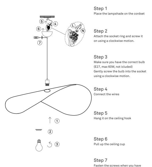
adjusted the cable to desired length.
